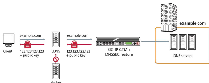
Figure 2: BIG-IP GTM DNSSEC feature interaction
