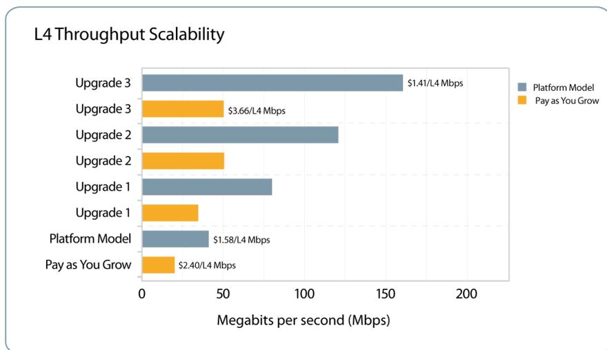
**Figure 2:** The layer 4 throughput of a pay-as-you-grow (licensing-based) scalability model increases at a slower rate and higher per-transaction cost than in a platform-based (hardware) scalability model.
