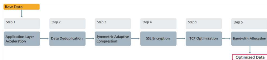
Figure 6: How BIG-IP LTM with BIG-IP AAM optimizes applications and data transfers
