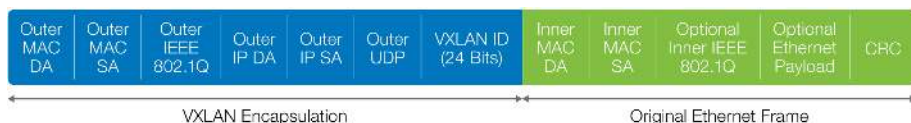
Figure 3: VXLAN extends standard Ethernet frames, enabling the coexistence of virtual networks with traditional IP networks.
